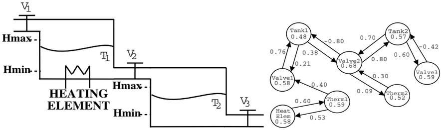
Fig. 1. The process control problem (left) and the corresponding FCM (right).
